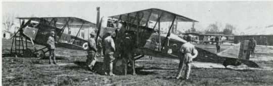
Interesting view of 87 a Sq. S.V.A.s on a forward airfield. The aircraft in the foreground carries three bomb clips on the port side.
