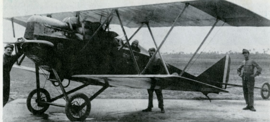
An Isotta-Fraschini-engineered S.V.A.5 during early post-war airmail experiments. The bags were strapped to the fuselage above decking, with severe results to the pilot's forward vision! (Photo: G. Apostolo via the author)
