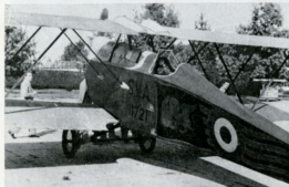
An S.V.A. in the (probably spurious) markings of the 87 a Squadriglia; note instrumentation and twin auxiliary petrol tanks on the upper wing centre-section. (Photo: the author)
